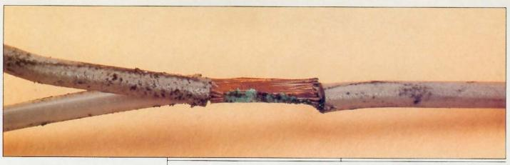
wire ties; they can work loose and be cut or broken during mechanical repairs. Loose harnesses can chafe against bulkheads or other machine parts, wearing away their protective covering and making their wiring susceptible to corrosion. They also can dangle in the way of moving parts, which can sever them and cause a short circuit. "Short circuits are the most damaging of all electrical failures," says Vaught. "They leave the circuit unprotected and lead to machine fires."
